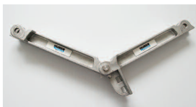
The chain forms its own frame! It works similar to a knee or elbow.
